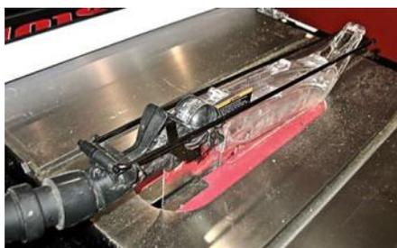
**Cross cutting** – This issue was brought to my attention by Craig Arnold, Director of Sponsorship and Shop Foreman. Proper procedure when using a sled is to install the sled on the saw with the blade lowered completely into the table. In similar fashion, lower the blade completely when you have completed your operation and prior to
