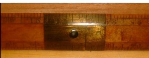
sand and clay which acts as a binder. The pattern is removed and the depression remains. The cope and drag are put together. Molten metal (brass, iron, bronze, aluminum) is poured into the mold, at the foundry. Each of these metals shrinks in the mold on cooling to their final specifications. Since each metal shrinks a different amount a different shrinkage rule for each type metal has to be used to create the pattern. There were no shrinkage rules in Fred's toolbox. However, Fred did make a
