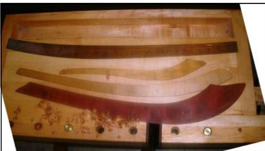
Fred also made sweeps and straightedges of nice thin pieces of figured maple or of the same red composite. Sweeps are like rulers, some marked off by hand in inches, some not, that make gentle curves in three dimensions. They are thin and flexible and allow the drawing of gentle curved lines on flat or three dimensional surfaces (think drawing a curved line on a globe's surface).
