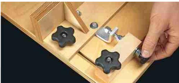
The router table in my shop gets lots of use. But it's always difficult to make fine adjustments to the fence. So I built the micro-adjuster you see in the photo above using spare parts I had around the shop.
