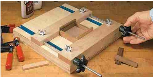
When gluing and clamping small parts together, it's always a challenge to align large clamps to hold them in place as the glue dries. To make this job easier, I built the small parts clamp you see in the photo above.
