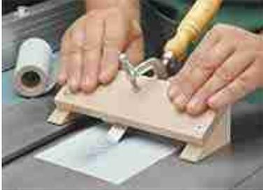
I use sandpaper to sharpen my chisels. By “sanding” the bevel of the blade flat and smooth, it produces a sharp edge in just a few minutes.
