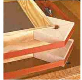
Whenever I glue up a case, it’s always a challenge to spread the glue in the joint, assemble and square up the parts, and then install the clamps before the glue sets up. To make the job easier, I made a set of large corner clamping blocks, like you see in the photo at the right, to use with band clamps.
