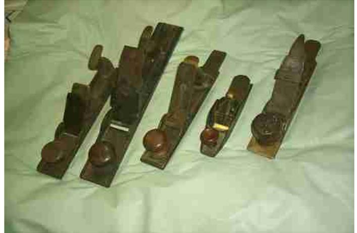
The patent papers for the first plane state that the width of the throat may be changed by placing the wooden wedge either behind or in front of the blade.
