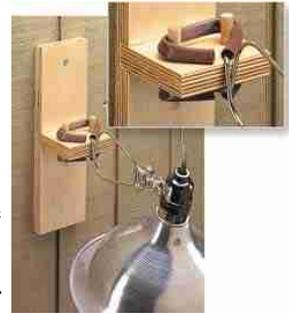
To solve this problem, I devised a holder for my shop that can be placed almost anywhere. This holder allows the lamp clip to grip securely so I can have constant and stable light at all times.
