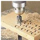
**1.** With a plug cutter chucked in a drill press, cut the plugs in a scrap piece from the project. Be sure to make a few extra. This way, you'll be able to select a plug that best matches the color and grain of your project.
