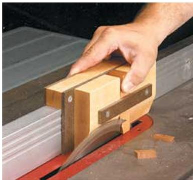
It's made by gluing and screwing two hardwood supports to a 1/4" hardboard front, as in the drawing. (Note: Make sure the screws are located above where the
