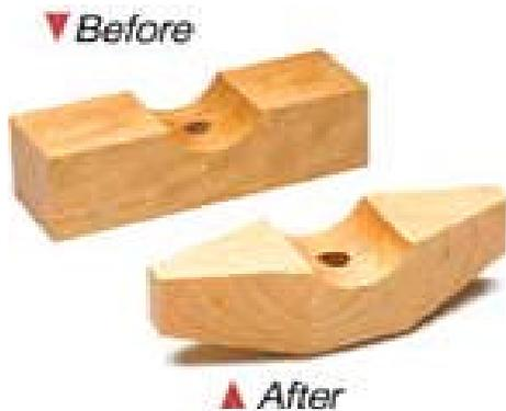
The jig rides on the rip fence and holds the blanks in place while they're being cut. It's de-
