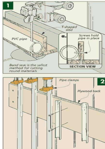
section of PVC pipe to set the band saw fence. You want the clamps to snap easily into place but with enough "grab" to hold them firmly.
