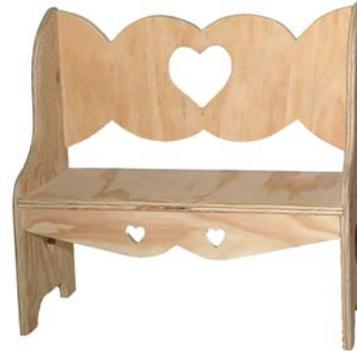
**Kevin McAndrew's** child's bench made of plywood, as yet unfinished. The challenge was to cut out the small hearts. The tools used were a table saw, coping saw, jig saw and Dremmel tool.
