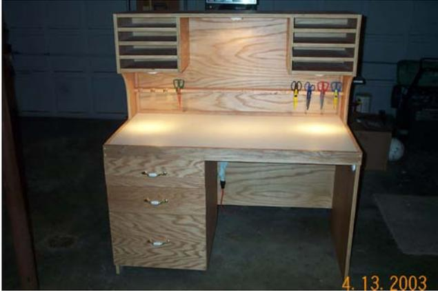
**Trent Glamann's** scrap booking desk made of 3/4" inch Oak Plywood. It was finished with wipe on poly, and has scissor hangers and recessed lighting. The challenge was the one piece sides.
