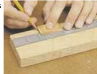
My solution is the simple rule guide shown here. It's a small wood block that makes it easy to accurately lay out a line. You simply align the end of the block with the desired increment on the rule. Then mark the line, using the block as a guide.
