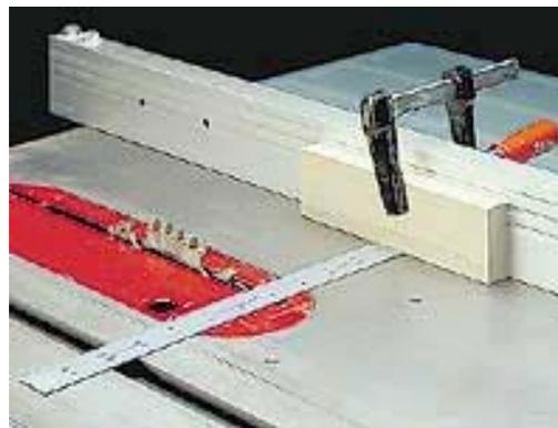
My set-up gauge consists of nothing more than a block of hardwood and a 12"-long steel rule, see drawing above.
