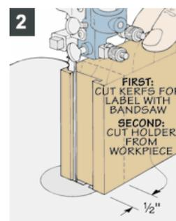
The recess is made in two steps. Start by routing a shallow groove in the edge of the work piece, as shown in Figure 1. Then, to create slots that "trap" the label, use a band saw to cut two thin kerfs in the corners of the groove (Figure 2 and detail below).
