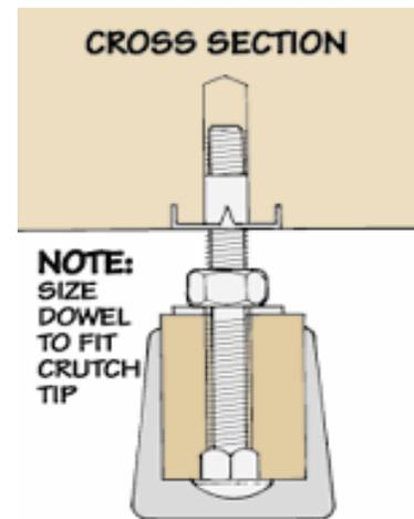
for the bolt as you adjust the leveler, you'll need to drill a deep shank hole for the T-nut, as shown in the Cross Section drawing above.
