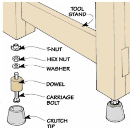
over a dowel that has a hole drilled in it to accept a carriage bolt, as you can see in the drawing at left.
