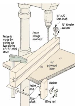
One end of the fence is attached to a plywood base with a carriage bolt and a threaded knob. This allows you to swing the fence in or out. The "free" end of the fence is then secured to the
